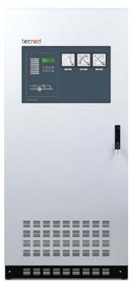
The TECNED-OM series is designed with reliable and robust IGBT-technology using analog monitoring and control circuits to minimize sensitivity to electromagnetic distortion. The high frequency controlled inverter is able to supply non-linear loads with minimum output voltage distortion, providing a constant voltage to the load under all operating conditions.
